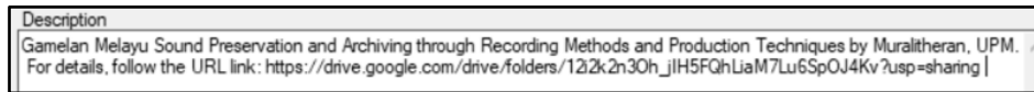
Figure 21: BEXT information in file attributes of the said wave file and this information retrieved by using Steinberg Wavelab (photo by the author).
